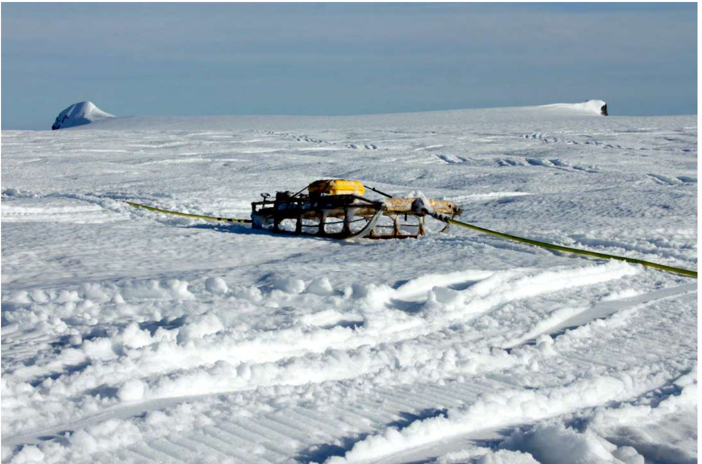
Radio-echo sounder on Öræfajökull volcano - near southern edge of Vatnajökull Glacier
